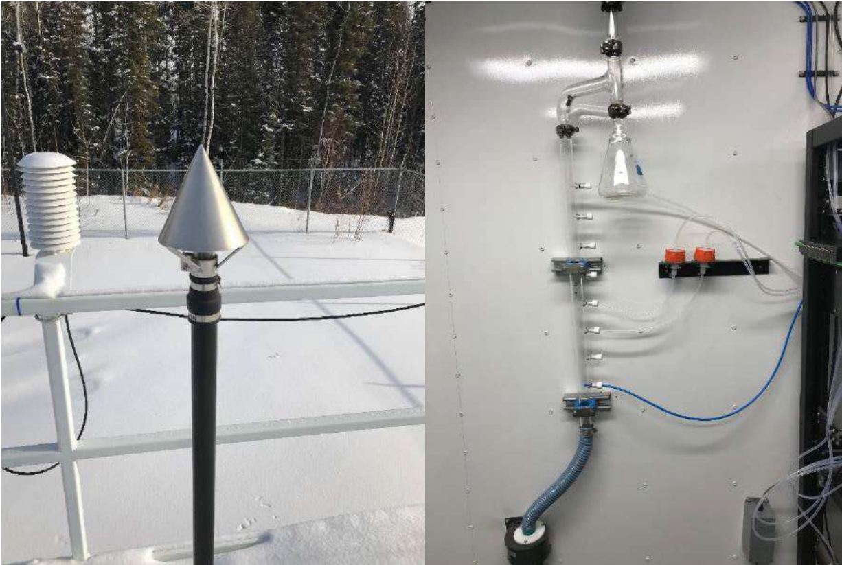
Figure 7.0 – Photo showing the inlet and sample manifold
