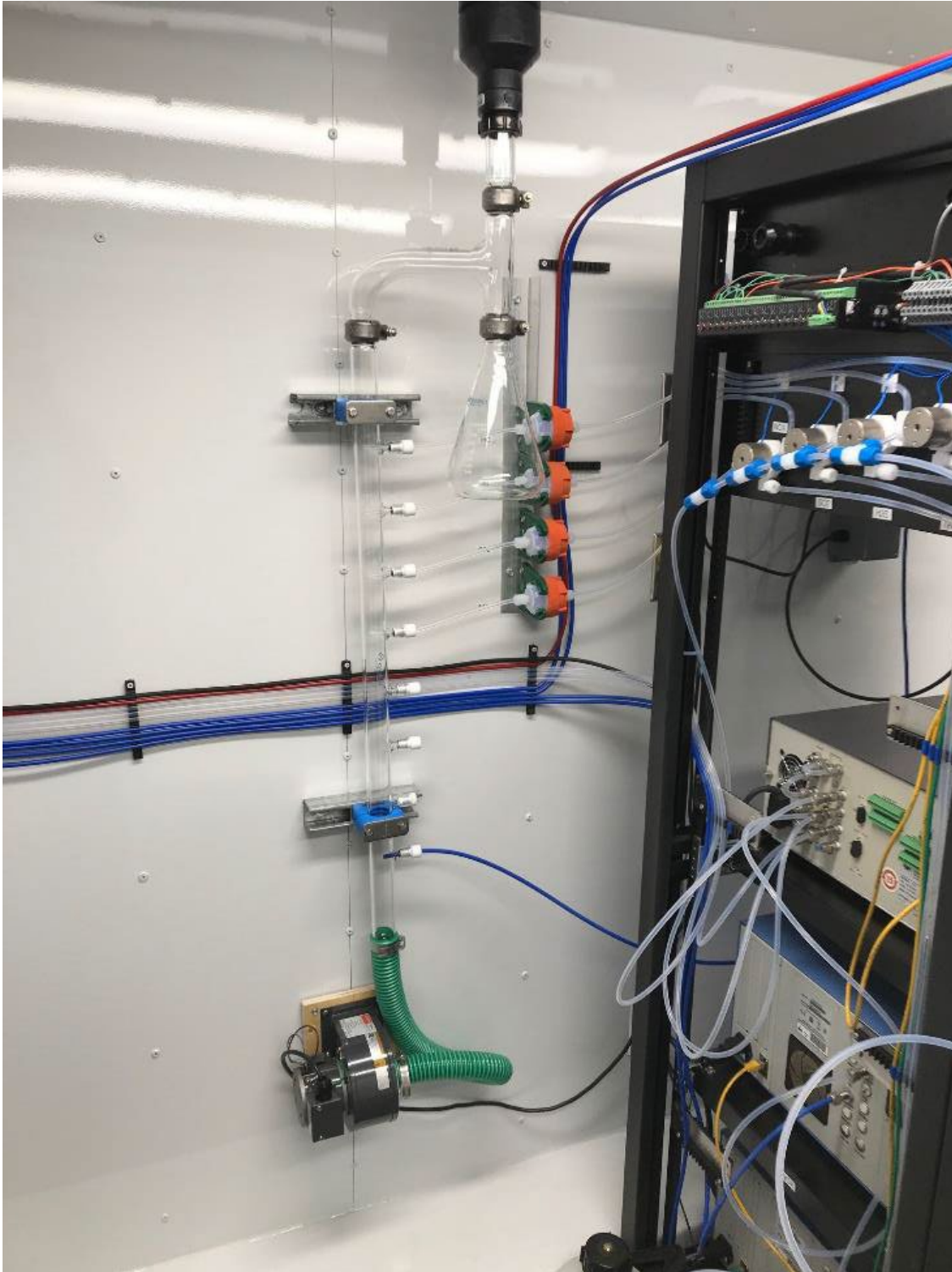
Figure 9 – Photo showing the inlet and sample manifold
