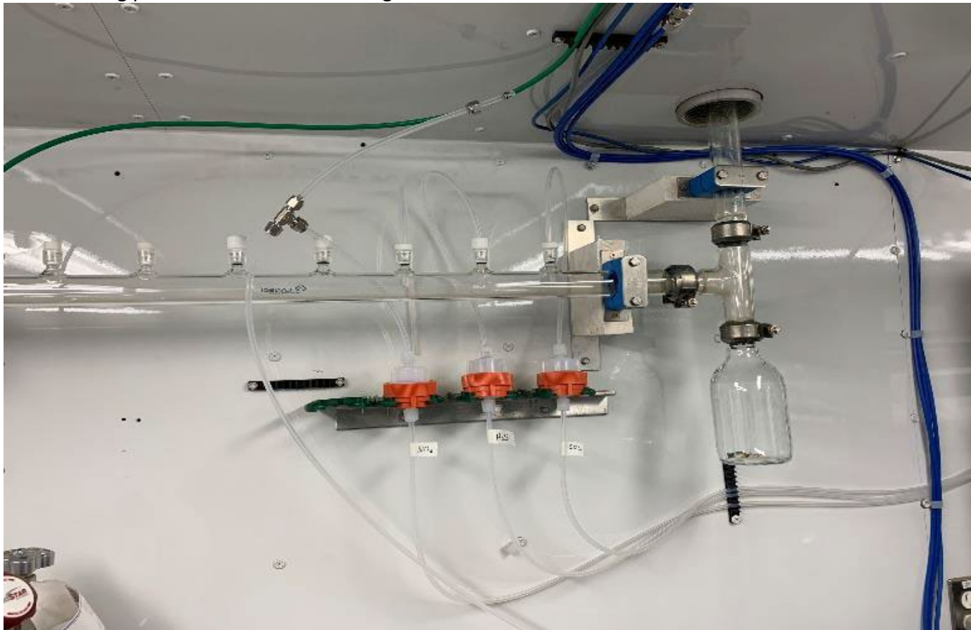
Figure 9 – Photo showing the inlet and sample manifold.
