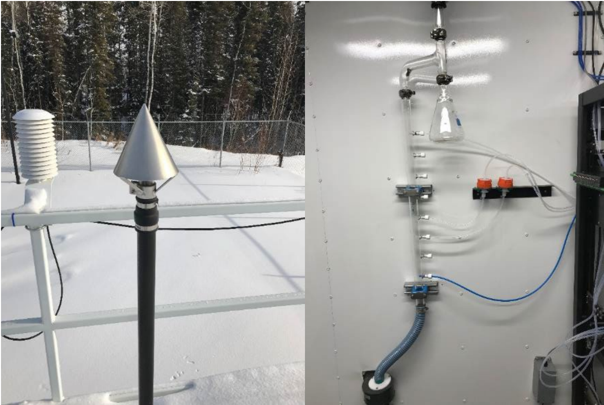
Figure 10 – Photo showing the inlet and sample manifold
