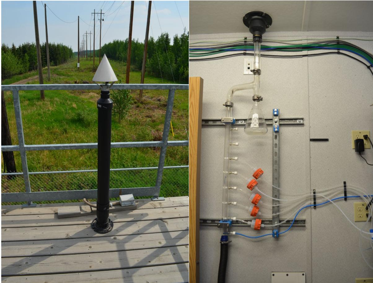
Figure 10 – Photo showing the inlet and sample manifold
