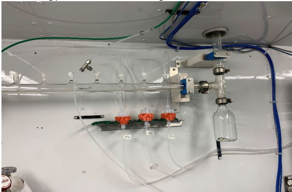
Figure 6.0 – Photo showing the inlet and sample manifold
