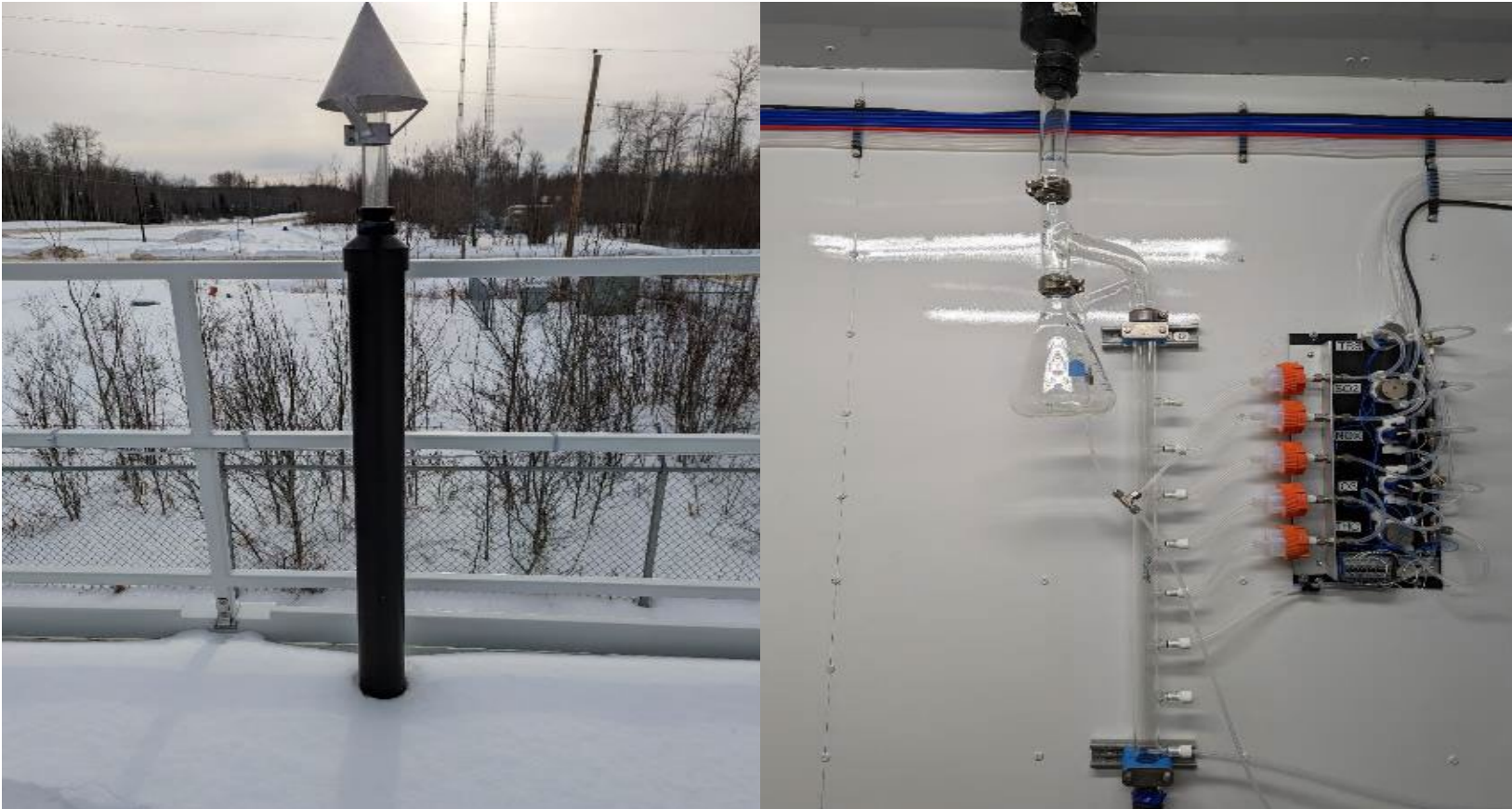
Figure 7.0 – Photo showing the inlet and sample manifold
