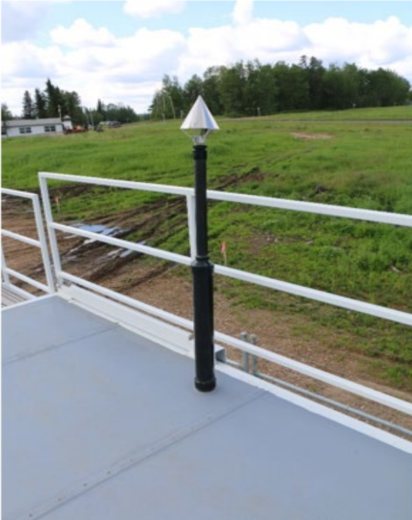
Figure 7.0 – Photo showing the inlet and sample manifold.
