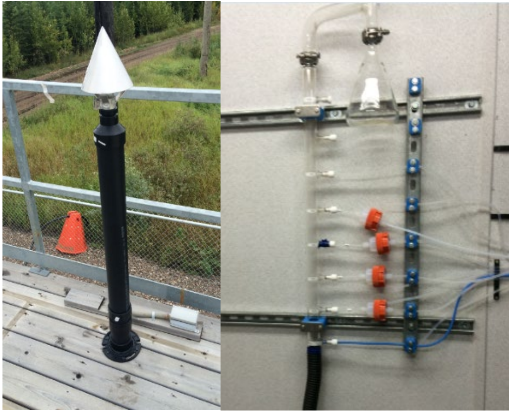
Figure 7.0 – Photo showing the inlet and sample manifold
