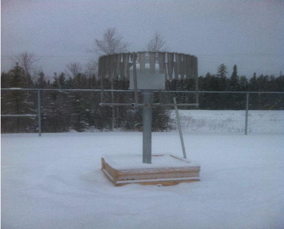
Figure 4.4– Continuous precipitation monitoring instrument (Pluvio)
