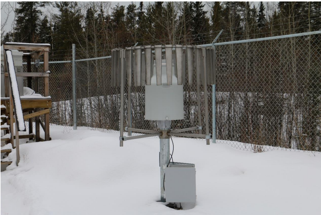
Figure 4.5 – Continuous Precipitation Monitoring Instrument (Pluvio)
