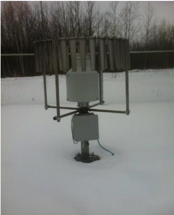
Figure 4.10 – Continuous precipitation monitoring instrument (Pluvio)
