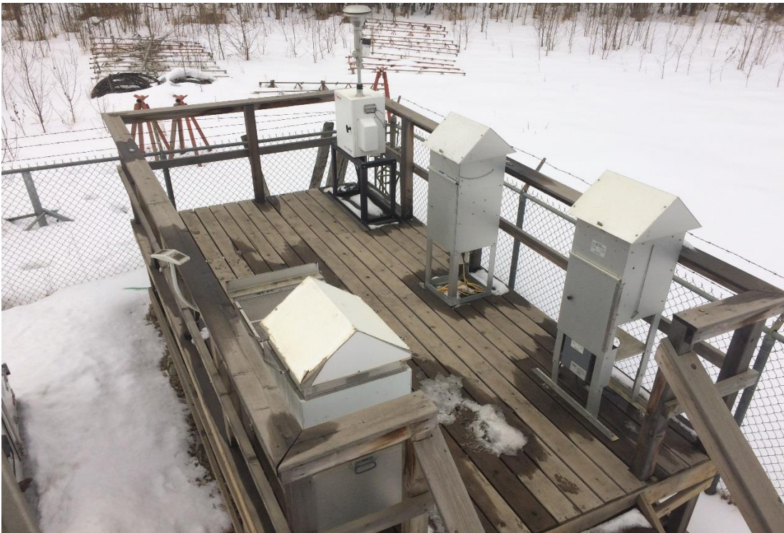
Figure 4.1 – Sampling deck which contains EC PM2.5 Partisol sampler & EC High Volume PAH sampler
