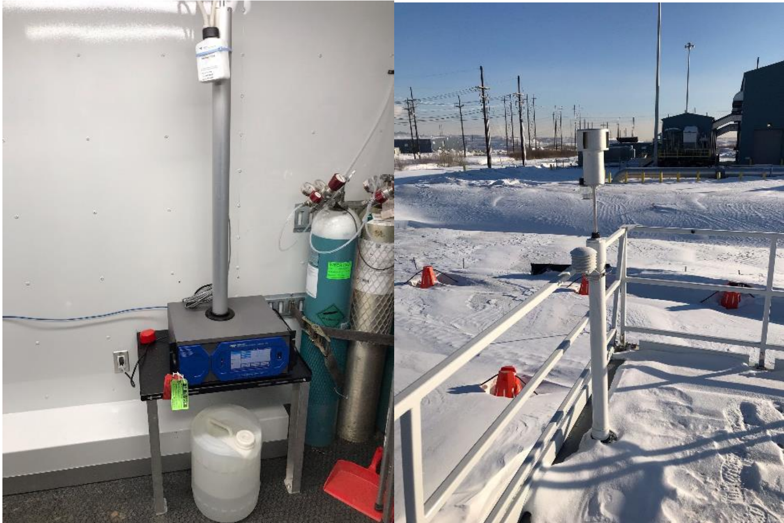
Figure 6.3 –Photo of the T640 PM monitor and inlet
