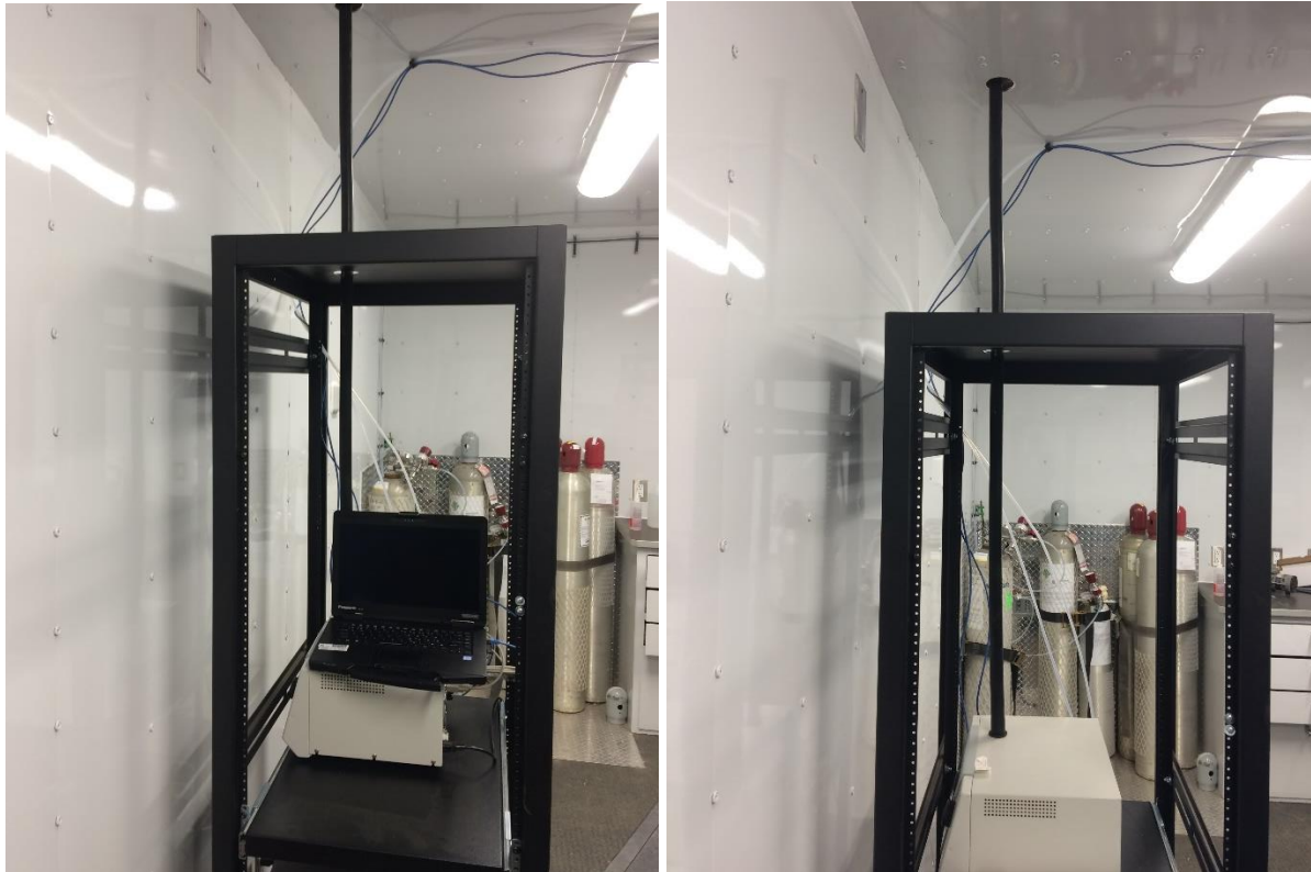
Figure 7.3 –Photos of TSI Particle Counter
