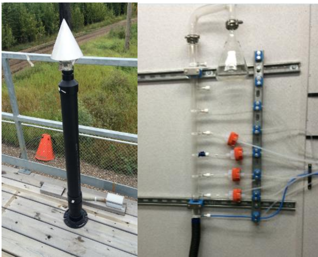
Figure 7.0 – Photo showing the inlet and sample manifold
