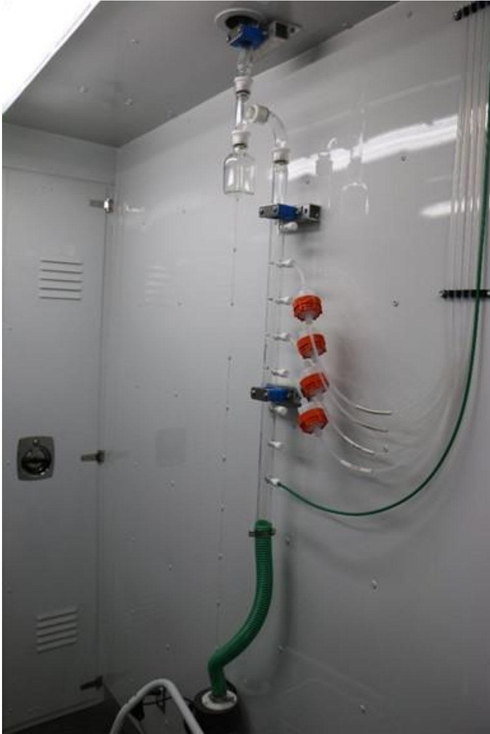
Figure 6.0 – Photo showing the inlet and sample manifold
