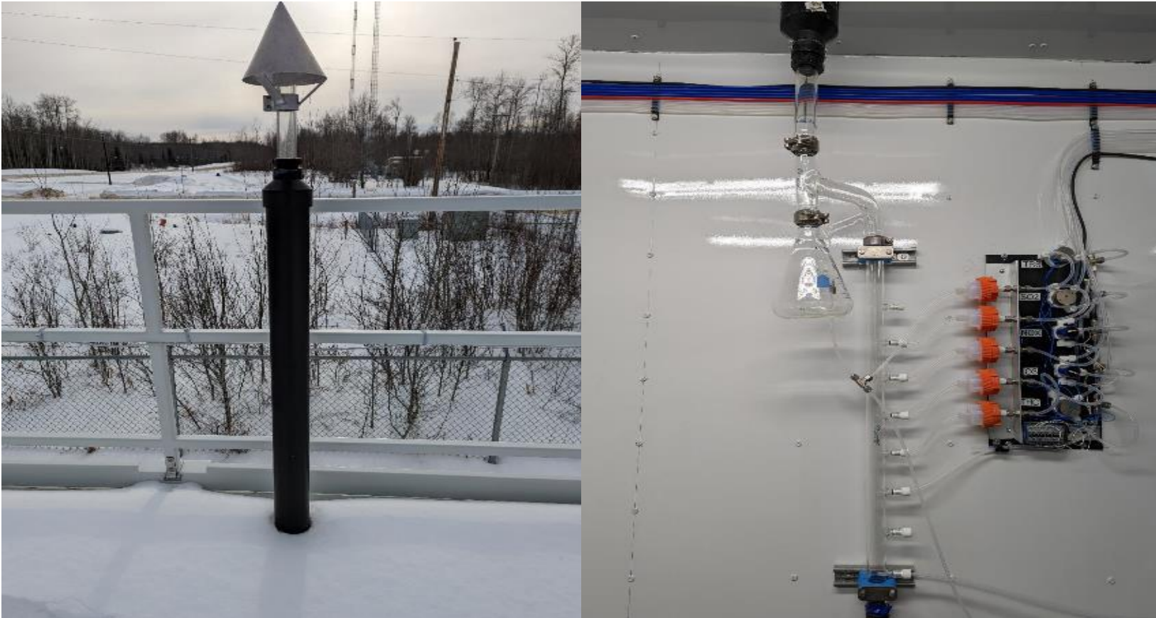
Figure 7.0 – Photo showing the inlet and sample manifold
