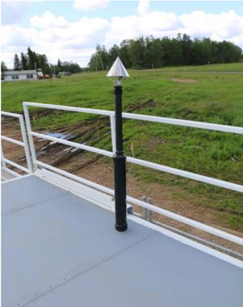
Figure 7.0 – Photo showing the inlet and sample manifold.
