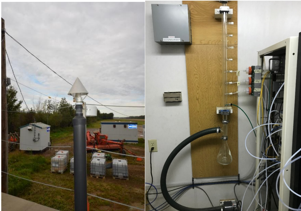
Figure 6.0 – Photos showing the inlet and sample manifold
