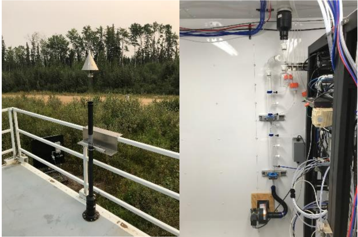
Figure 6.0 – Photo showing the inlet and sample manifold
