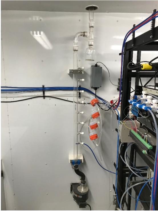
Figure 6.0 – Photo showing the inlet and sample manifold
