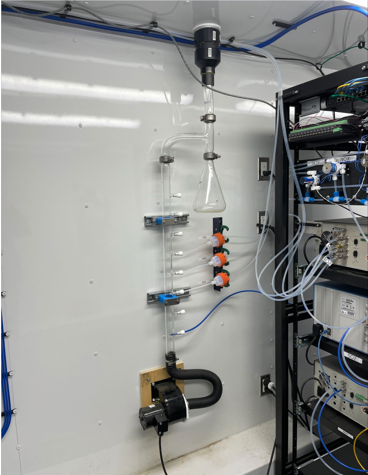
Figure 7.0 – Photo showing the inlet and sample manifold.
