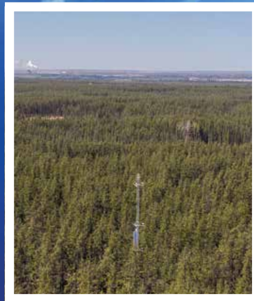
One of WBEA's five instrumented 30 m towers. This tower is located at WBEA Forest Health site JP104, located NE of Fort McMurray. These towers provide continuous meteorological and site-condition (e.g., light intensity, soil moisture) data, necessary for proper interpretation of air quality and ecological monitoring data.
