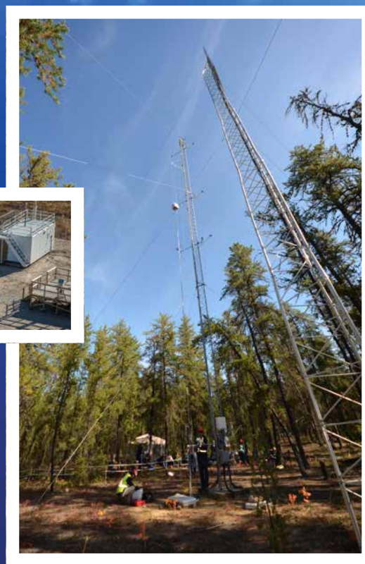
WBEA members observed the change out of passive air pollution filters, situated on the tall meteorological tower at forest health site JP104, during the Member's Open House.
