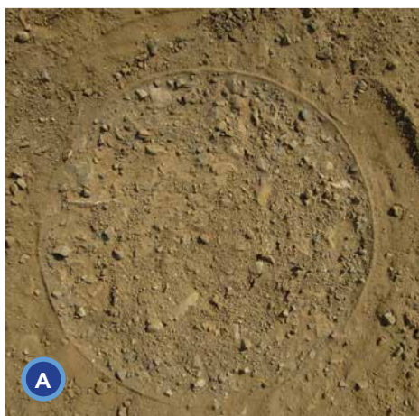
Figure 6. Two different unpaved surfaces show large variation in fugitive dust emission potential for: a) a heavy hauler road, the first stacked bar in Figure 5a; and b) a lightly traveled unpaved road without heavy vehicles, the fifth stack bar in Figure 5b. Note the smaller particle sizes of silt and clay in Figure 6a. The ring was created by the PI-SWERL.
