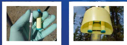
Figure 2. Radiello diffusive samplers. Left - adsorbing cartridge outside of the diffusive body; right - Radiello R145 and R141 assembled within their diffusive bodies and installed in a protective shelter.
