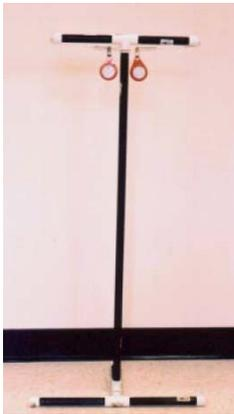
**Indoor and Outdoor Monitoring** – Each type of passive and active monitor is placed inside and outside a person’s home. A stationary stand is used to house the monitors during the seven-day monitoring period.
